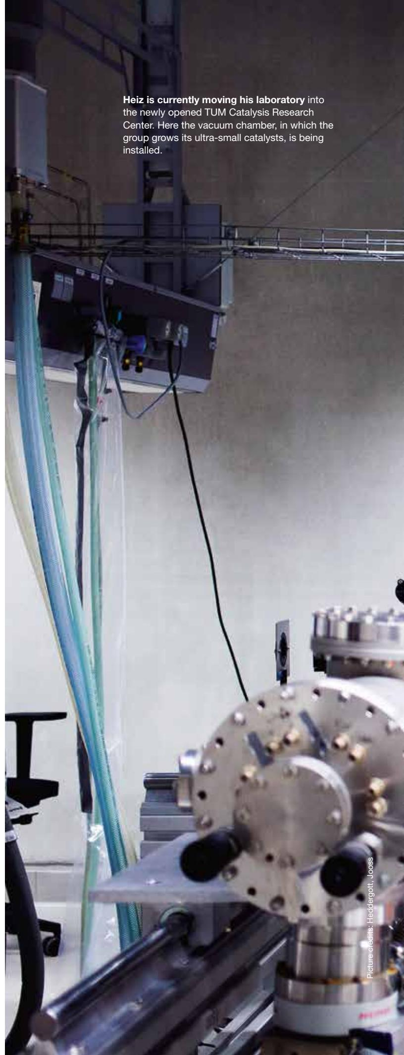
Heiz is currently moving his laboratory into the newly opened TUM Catalysis Research Center. Here the vacuum chamber, in which the group grows its ultra-small catalysts, is being installed.
