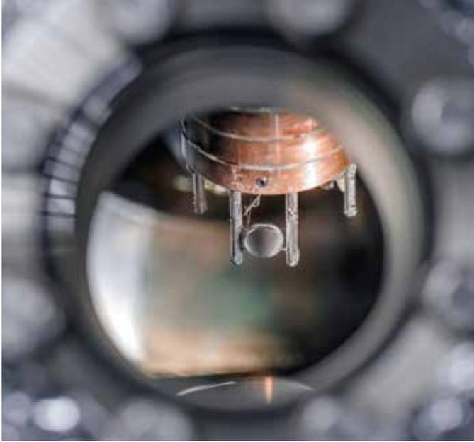
**Sample holder** with three single crystals on which the catalyst particles are deposited.
