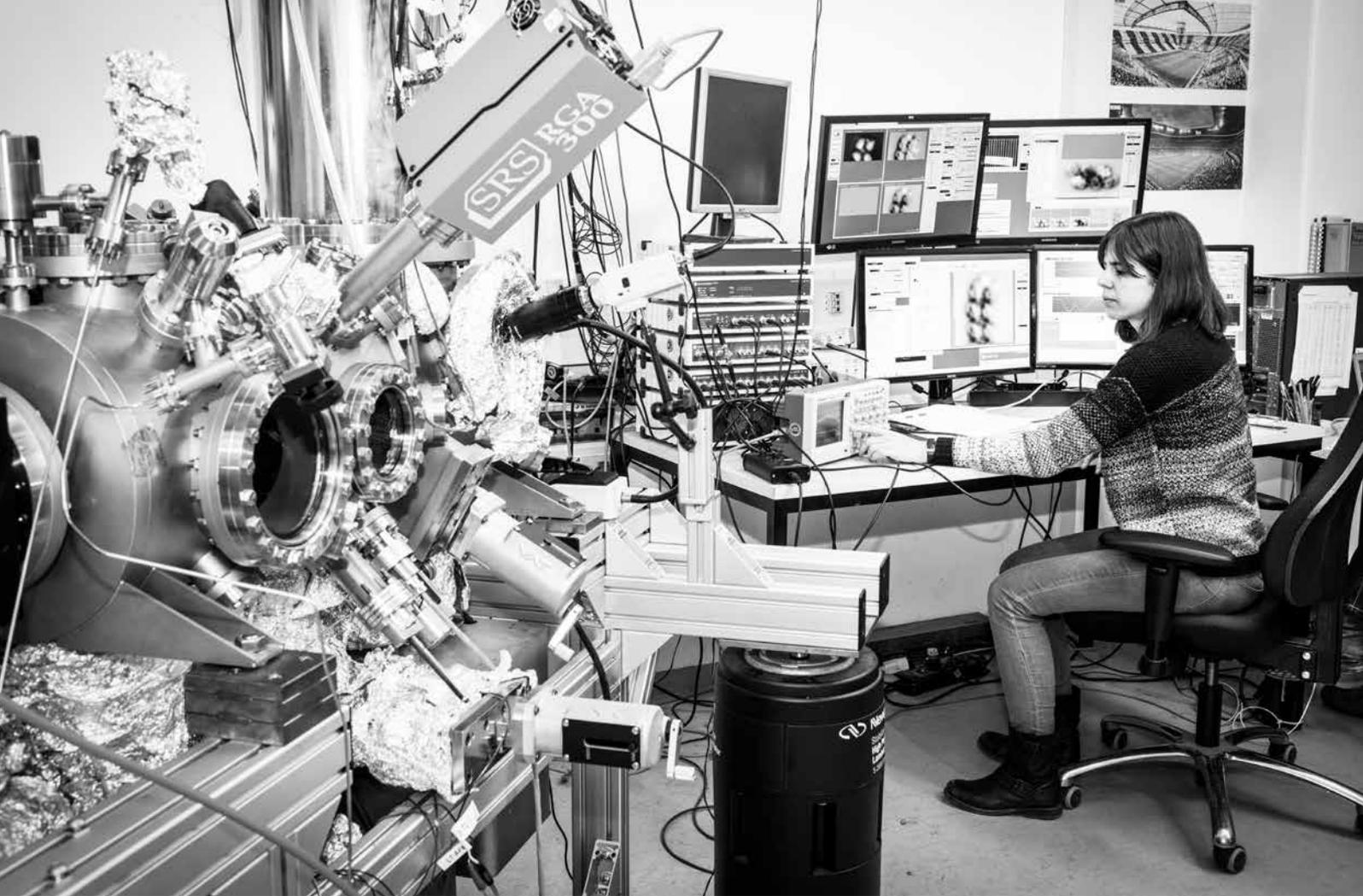
This combined scanning tunneling and scanning force microscope is used by the researchers to investigate molecular features and functionalities in unprecedented detail.
