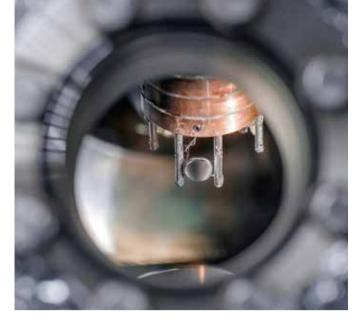
Sample holder with three single crystals on which the catalyst particles are deposited.
