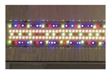
**Proprietary LED based lighting simulates** the different radiation intensities and spectral characteristics found in latitudes from the Baltic to the tropics.
