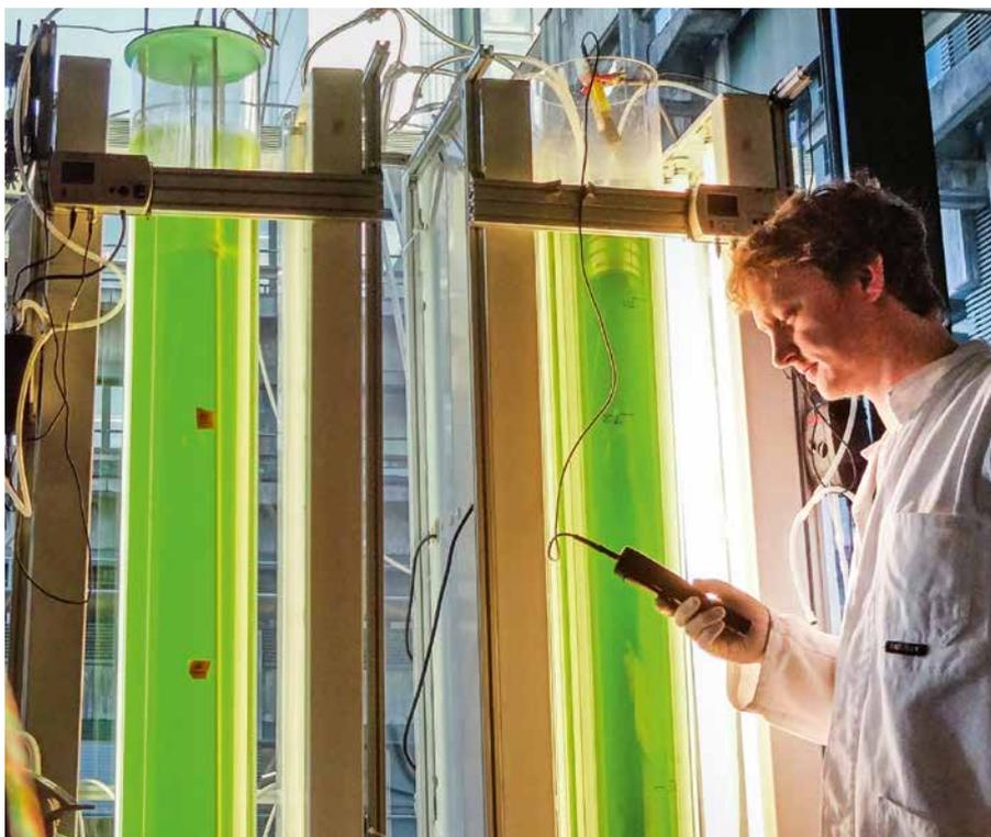
**The final laboratory-stage** algae process scale-up is realized in custom-built bubble column reactors holding 30 liters.
