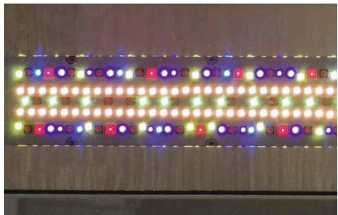
**Proprietary LED based lighting simulates** the different radiation intensities and spectral characteristics found in latitudes from the Baltic to the tropics.
