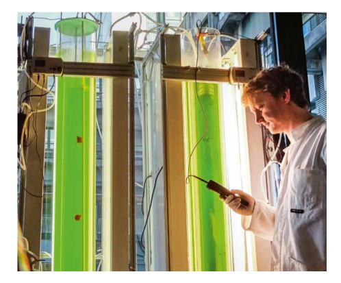
The final laboratory-stage algae process scale-up is realized in custom-built bubble column reactors holding 30 liters.
