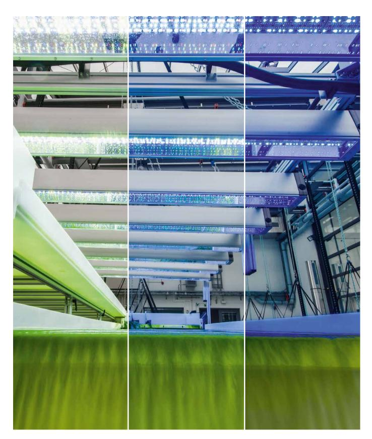
**The AlgaeTec Center allows simulation** of the climate and illumination of any potential production site. The Brück-led research consortium developed an optimized "cascade" cultivation system, which encompasses two small steps that have been incorporated into the 200 liter tanks. Gravity causes the algae cultures to flow down into the next-lowest tank. In the collecting basin at the bottom, the entire solution is re-saturated with CO<sub>2</sub> and then pumped back up to the highest level.
