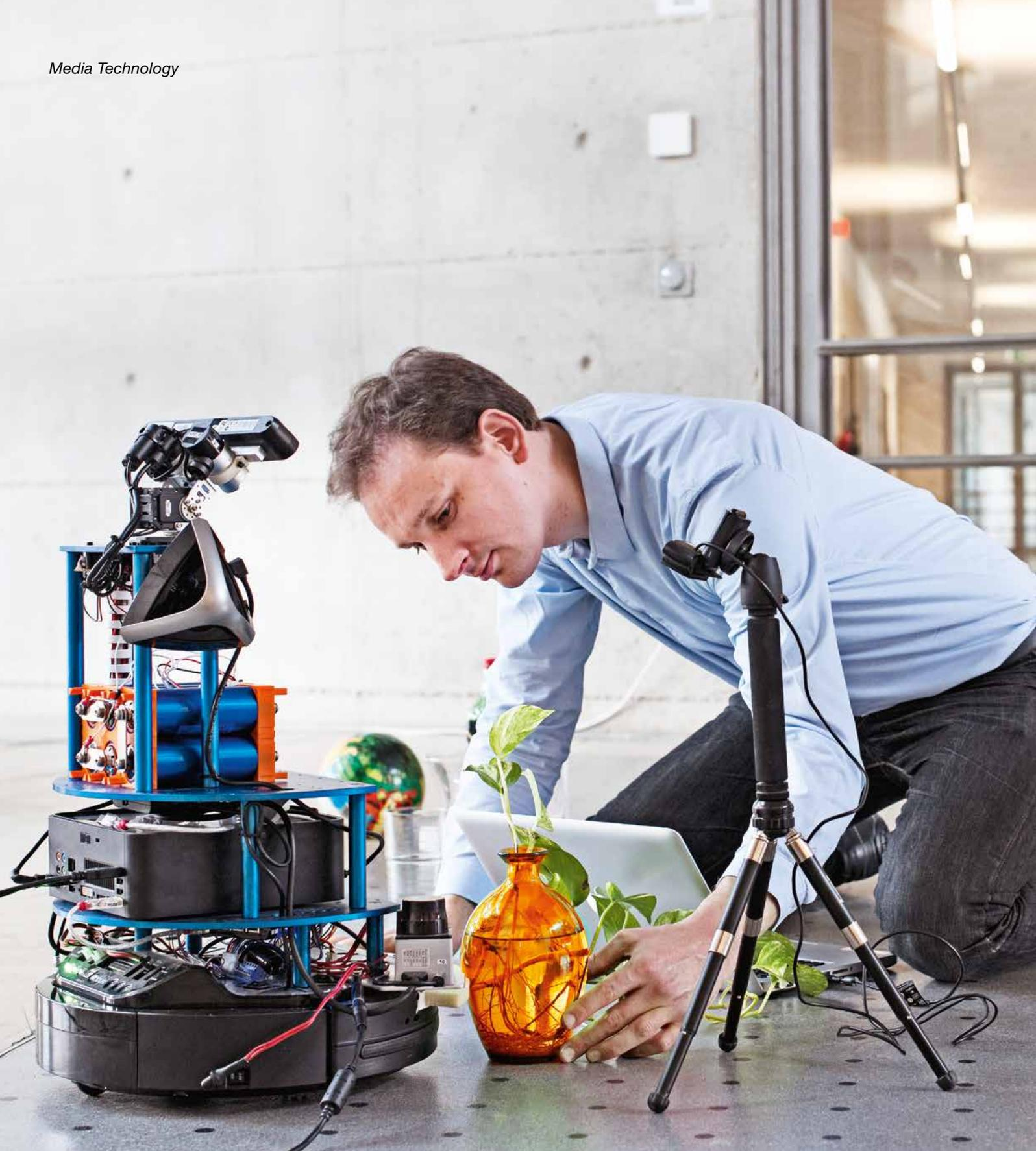
Vacuum cleaning robots normally use **infrared** beams to scan their surroundings. But that does not always work with transparent objects. This robot is equipped with a type of plastic bumper. A camera monitors deformation of the plastic.
