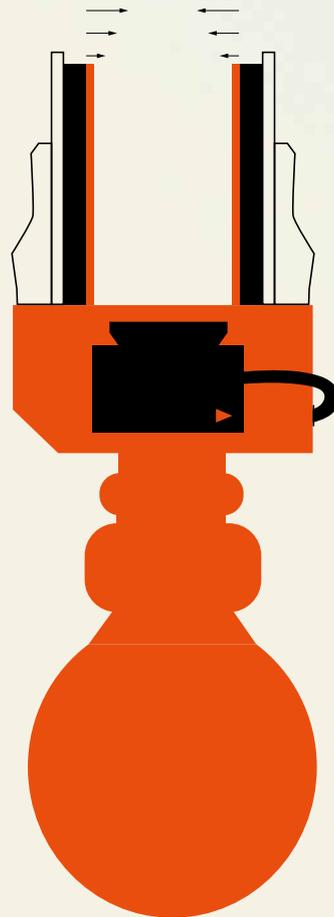
**Robots can precisely grasp firm objects** but pliable objects still pose a challenge – unless they are equipped with force and pressure sensors. The ROVI system determines the force from the deformation of gripping jaws made of rubber, which is picked up by a camera.
