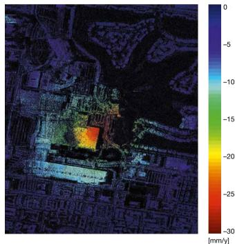
**Monitoring subsidence:** The top image is a TerraSAR-X view of Las Vegas Convention Center and an adjacent golf course. The bottom image shows ground subsidence of up to 3 centimeters per year caused by withdrawal of ground water near the Convention Center between 2009 and 2010. Radar interferometry is used to measure many subsidence phenomena, e.g. in former mining areas or the effects of gas extraction, oil pumping or subway construction.
