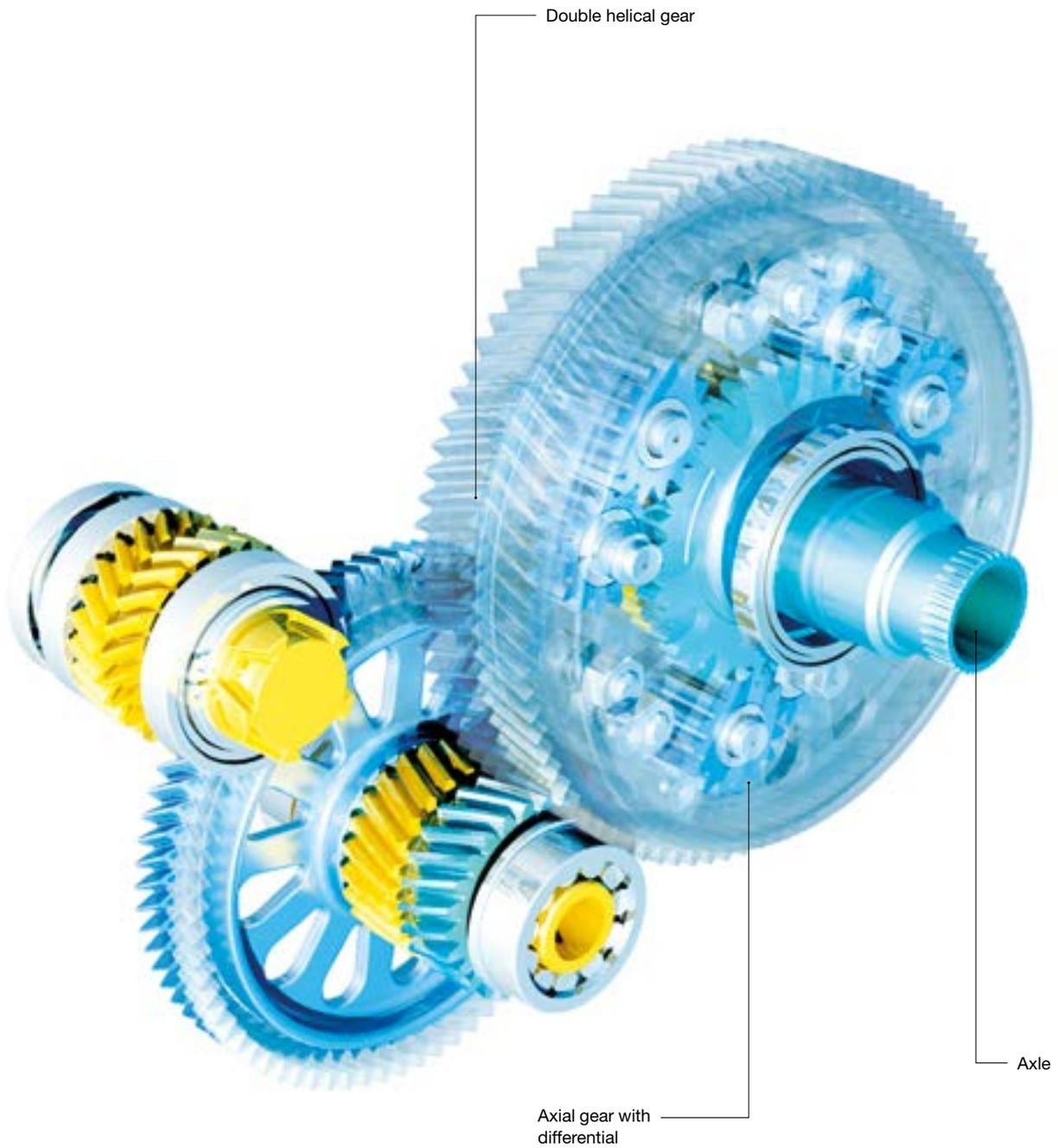
In order to realize a plastic housing for the torque vectoring unit, the TUM engineers had to find a way to reduce the forces of the gear system. They overcame this challenge by designing a double helical gear, in which the axial forces cancel each other out.
